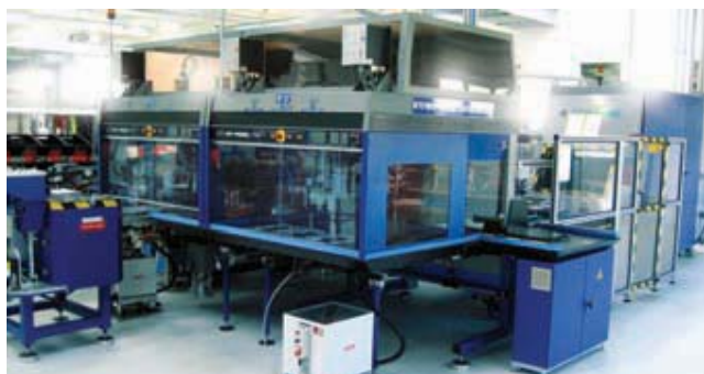
Up-to-date production: production takes place on five active carbon lines in two shifts on new knife pleaters as well as a folding and strapping machine.
