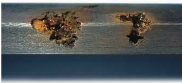
Cavities at the cylinder liner: after the liner has been cut open it can clearly be seen that the cavities are becoming larger towards the inside.
